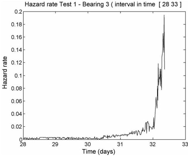
Fig. 10. Hazard rate prediction of bearing 3 in test 1.
