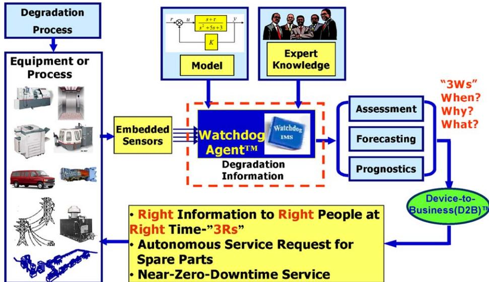
Fig. 1. Infotronics structure of IM systems.
