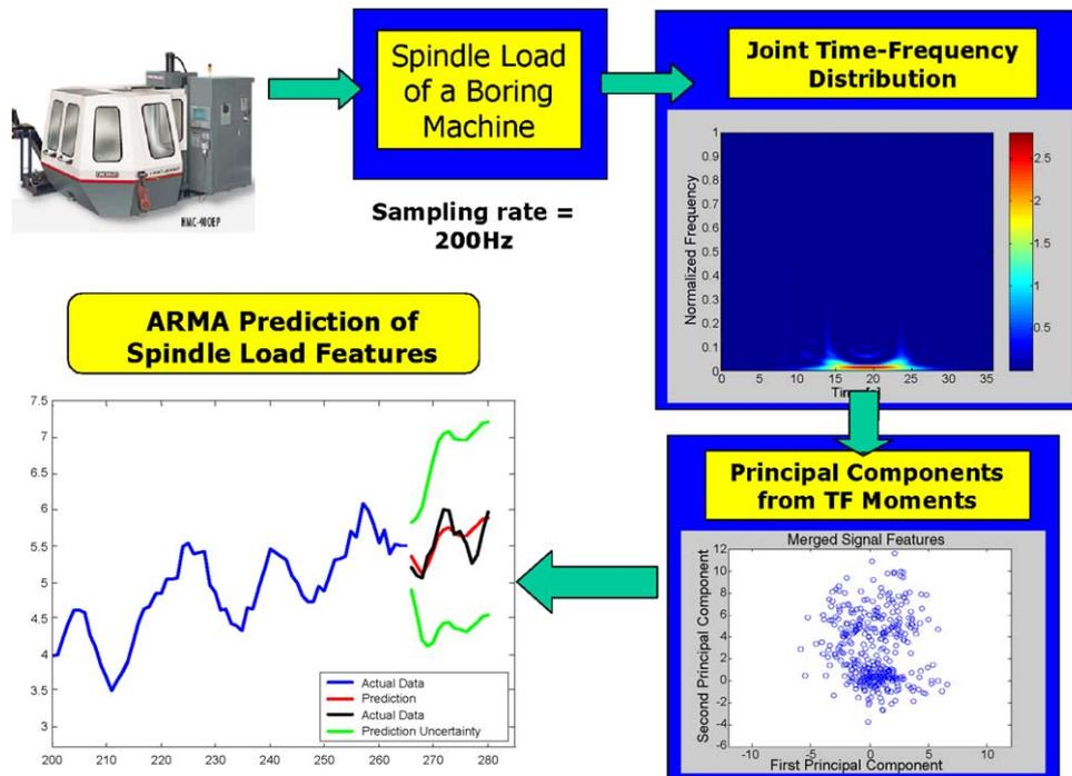
Fig. 6. ARMA prediction of features extracted from the spindle load sensor readings.
