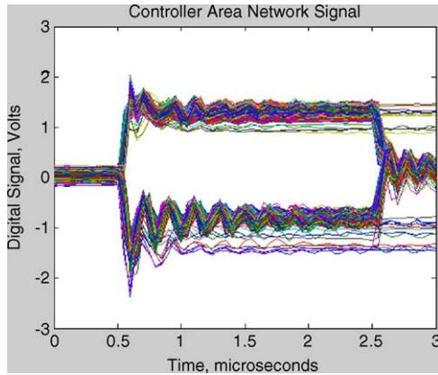
Fig. 11. Time series data for CAN Network.
