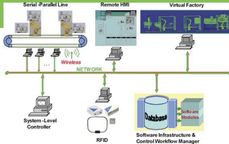
(HMI) to provide connectivity for diagnostics, maintenance, and order placement, utilizing data gathered from sensors/machines using OPC and XML. These web-based tools also give researchers and industry partners access.
